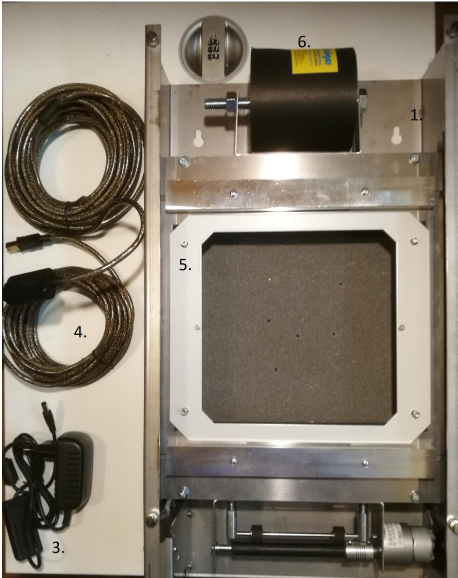
Picture 1. Composition of InBand electronics scoring target
